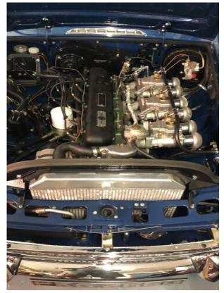
Experience to date has been limited. There are a few snags, which will be sorted over the next week or so, but I am really impressed with the rock steady idle at **750rpm**, the engine was run-in on a testbed and produces **circa 190bhp** with **160–170 ft-Ib** of torque. **Kevin Whitehead**.
