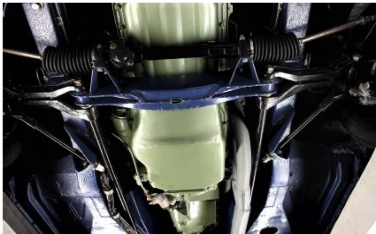
The MGC sump has to be extracted around the suspension cross member that's welded to the chassis
