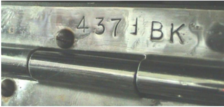
Chassis number stamped on bonnet hinge - quite rare on Triple-M cars these days.
