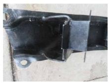
Sometimes these MGC mounts are not available and MGB mounts can be used with slight modifications to the cross member. The gearbox mounting bolts and flanges are exactly the same as the MGC.
