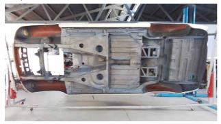
Sandy Beige and then white, but on the outside only. The car is now completely finished in white, a job done by **The Surgery in Wellington**. The underside of the car was finished in a two-pack white to match the body colour
