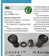
is incorrectly displayed in the original workshop manual. This will increase the pressure, putting extra load on the camshaft and distributor
